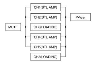
Note: • Connect both S-V<sub>CC</sub> and P-V<sub>CC</sub> to the power supply system externally. • Connect both S-GND and P-GND to the ground system externally.
